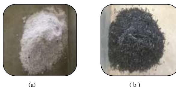
Figure 1. (a) Unprocessed NRHA and (b) Unprocessed BRHA
